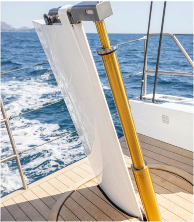
Double acting telescopic cylinder in titanium for rudder up and down.
