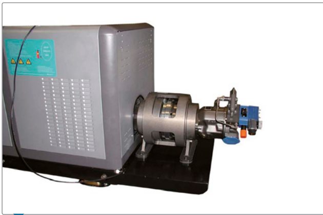
Pump assembled with custom clutch on 27kW generator PTO. Flow rate = 67,5 lit/min Max pressure = 250 bar.
