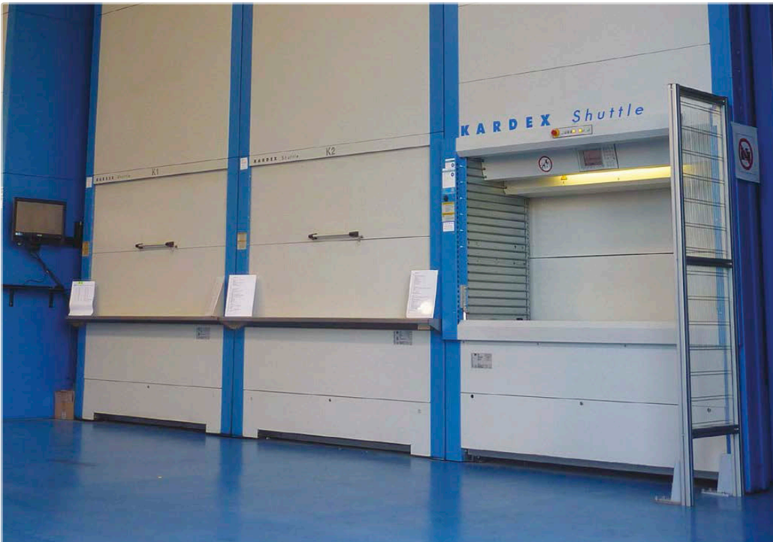
Kardex. Automatic warehouses. Seals, parts and tested products are all stored here managed by a software.
