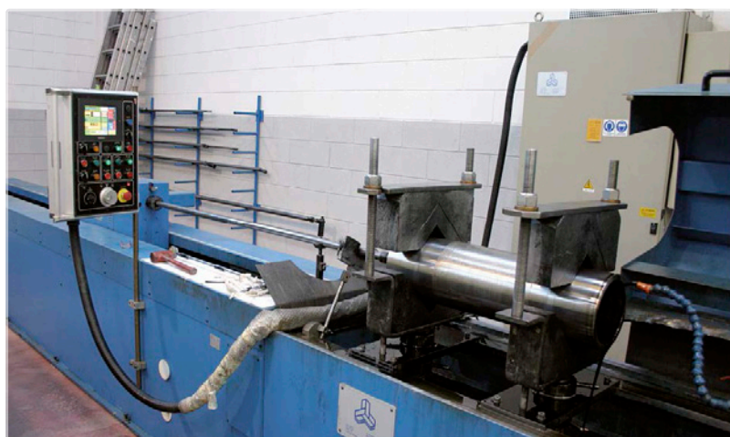
The "Lappatrice" is our CNC lapping machine used for every type of cylinder or Magic Trim tube. It can handle up to 4.5 meters of tube with an internal diameter of 400 mm!
