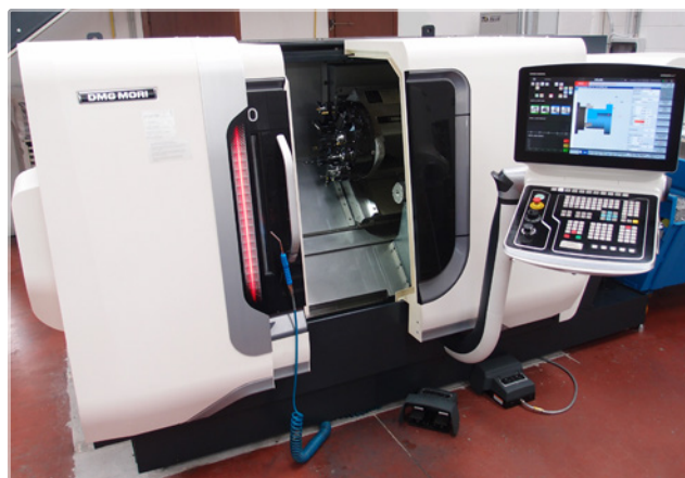
DMG Mori - CTX Alpha 500 - CNC lathe and milling machine, 4 axis. It is equipped with motorized tools, integrated mandrel motor and Y axis. It enables also off-center turning and milling.
