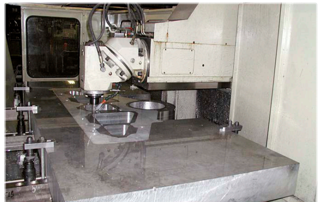
The "Tiger" CNC milling machine is one of the most reliable machines. The "Momac" lathe machine is used to produce small to medium pieces up to 400 x 1000 mm. Pins, small cylinder pistons and parts of manual components are machined here.
