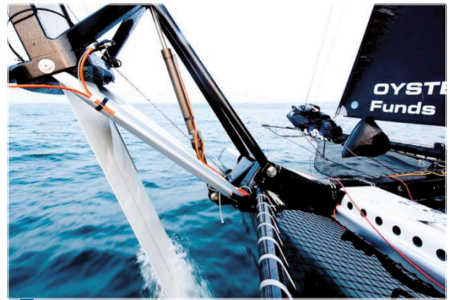
Double acting cylinder with integrated linear sensor to control foil angle of 32' race catamaran.
