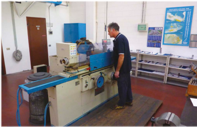
CNC grinding machine is used to machine the cylinders rods.
