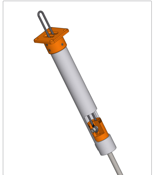
Inner forestay ram with lashing arrangement.
