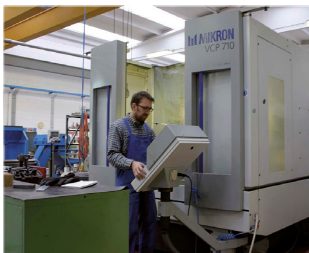
The "Mikron" small CNC milling machine is mainly used for the production of manual system components such as pumps, valves and other small parts. It is a 5-axe mill with a working space of 710x500x500 mm.
