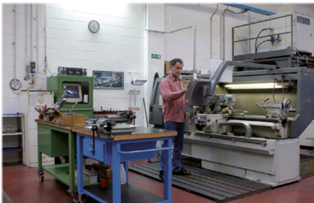
The "Momac" lathe machine is used to produce small to medium pieces up to 400 x 1000 mm. Pins, small cylinder pistons and parts of manual components are machined here.
