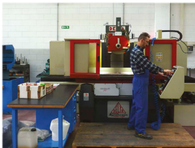
Grinding machine Delta compact plus X 1100 Y 600.
