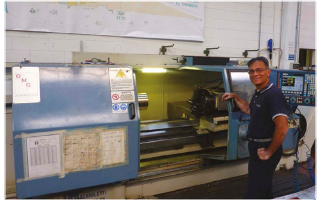
The "Zanoletti" medium size 5 axes CNC lathe. Small and medium size cylinder parts are machined here.
