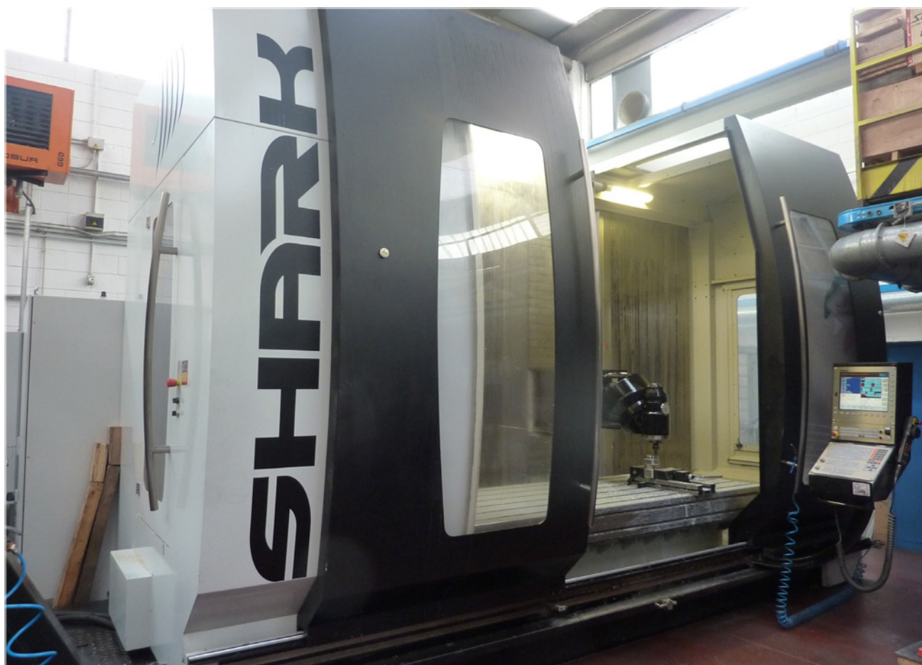
Shark milling machine Pieces are up to x 2500 y 1050 z 1200 mm.
