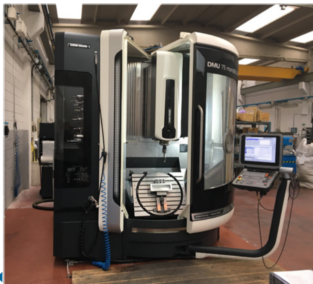
DMU 75 – Five-axis simultaneous machining with 750 mm X-axis traverse (75:750 mm), 20000 rpm speedMASTER spindle and a tool magazine with 60 positions.
