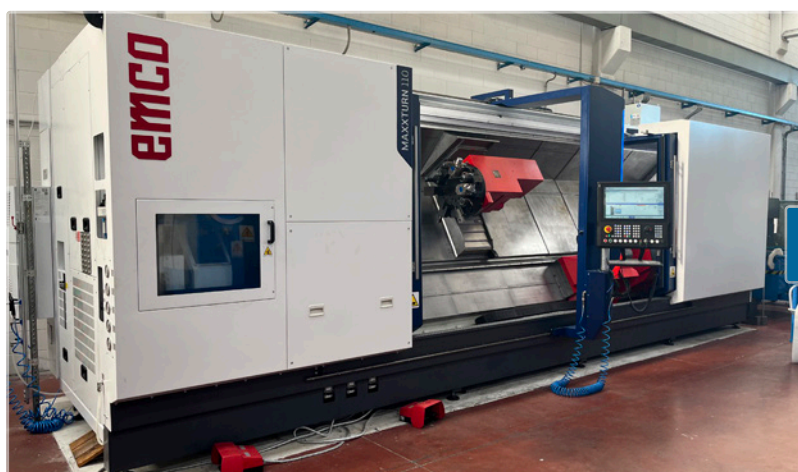
Emco Maxx Turn 110 – CNC lathe and milling machine, 4 axis. It is equipped with motorized tools, integrated mandrel motor and Y axis. Max Ø: 560 mm. Max length: 3520 mm.
