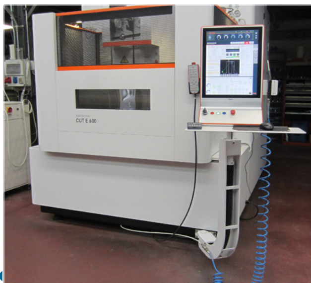
GF Machining Solutions CUT E 600 – With 600 X-axis, 400 Y-axis, 350 Z-axis, wire 0,25 mm max taper angle 30°/56 mm.
