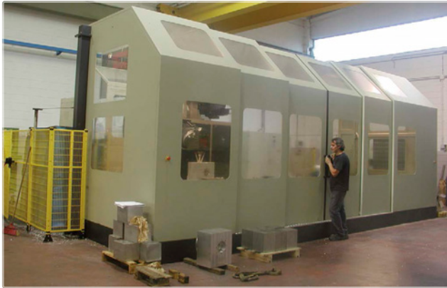
The "Tiger - TLM4" CNC milling machine is the biggest machine of the firm. The bi-rotating head works over a volume of 4000x1200x1500 mm and has a target power of more than 28 kW. Fins and bulbs are machined out here as are the biggest parts for the custom arrangements.
