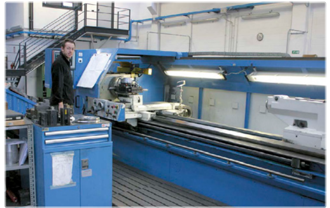
The "PBR" is the biggest lathe machine of the firm. It can machine tubes up to 3500 mm length with a diameter of 700 mm. Big Magic Trim tube, rods and big cylinders components are made by this machine.
