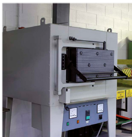
The oven for the heat treatment of special parts (like bolts for the canting keel systems). It can warm pieces up to 1100°C.
