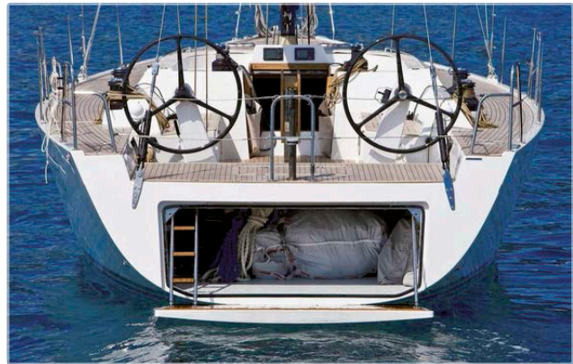
Solaris 48': customer rods link the transom door to the cars on the track of the Magic Door system
