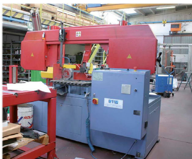
The chain saw cuts every size of pieces (aluminium, steel and titanium).
