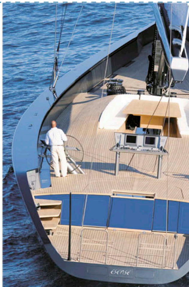
Wally 143; mainsheet and jib sheet are fully controlled by Magic Trim and Magic Double cylinders.
