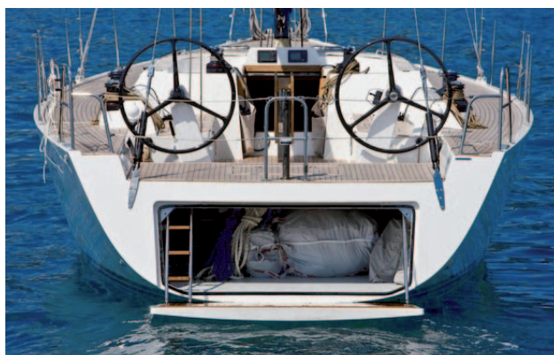
SOLARIS 48' "CRAZY TOO" (above): customer rods link the transom door to the cars on the track of Magic Door system
