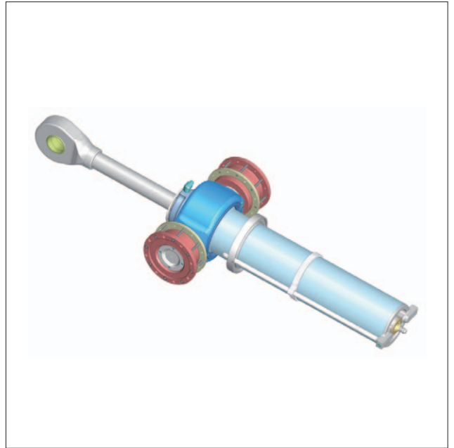
An OPEN 60 canting keel ram made of titanium
