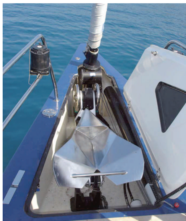
Anchor stowing motor
