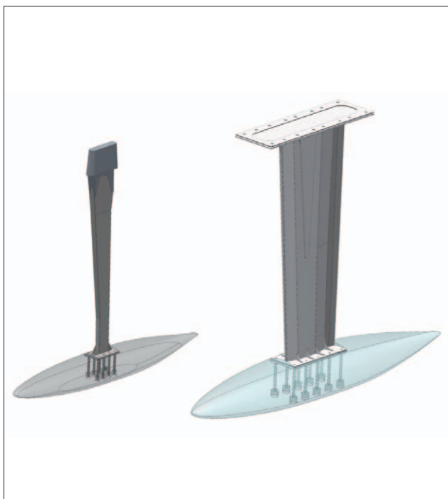
The fin on the left is CNC milling machined from a forged block to obtain the right shape. The one on the right is a welded fin made of Weldom.
